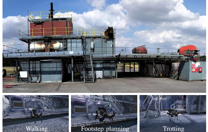
Fig. 1: A testing facility used for fire-fighter training, as a mock-up of an oil rig. Among other scenarios, we evaluate our method on this environment both in simulation and the actual location. The bottom row highlights different parts of a 25m long locomotion plan where 3 different modes of locomotion are required. The accompanying video presents the full experiment.
