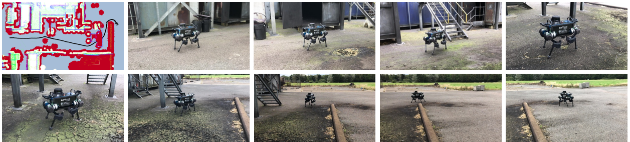
Fig. 9: Experiment 2 at the FSC oil rig. The first image shows the original cloud, navigation mesh, and executed path given by localization. The robot trots through the facility and around a 20cm barrier to reach a goal close its end.
